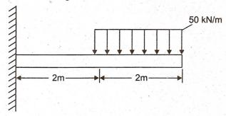
(b) Give the shear force and bending moment equation for the beam carrying the uniformly distributed load and concentrated load shown in figure. Also draw the shear force and bending moment diagrams.
