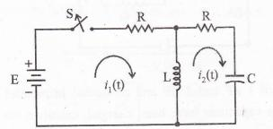
(b) For the circuit shown, the switch S is opened at t = 0. Use Thevenin's or Norton's theorem to determine the output voltage  $v_2(t)$ . Assume zero initial energy.
