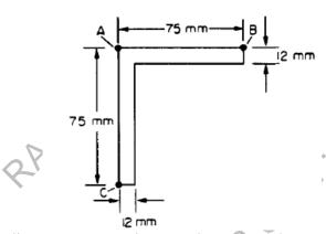
(b) The bending moment acting on the curved beam with a rectangular cross-section is M = 8 KN-m. Calculate the bending stress at point B.
