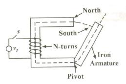
For an armature movement from open to closed position, find the magnitude of average magnetic force. The air gap length is 2 cm and the current during armature is constant at 40 A.
