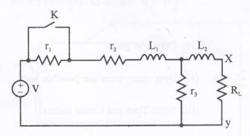
(f) In figure with switch open, steady state is reached with v=100sin314t volts. The switch is closed at t=0.
