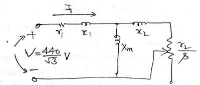
where  $r_1 = 0.294 \ \Omega$ ;  $x_1 = 0.503 \ \Omega$ ;  $X_m = 13.25 \ \Omega$ ;  $r_2 = 0.209 \ \Omega$ ;  $x_2 = 0.144 \ \Omega$ .
