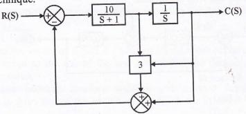
(b) Derive the relation for steady state error for the system of fig. 6. Also derive the value of steady state error for step input of magnitude A, ramp input of magnitude A and parabolic input of magnitude A.
