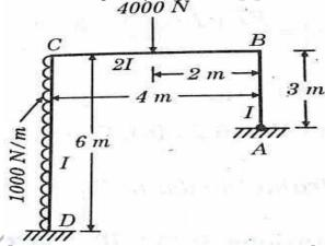
(b) Analyse the fixed beam shown in figure using strain energy method. And draw the B.M.D.
