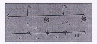
b. A fixed ended beam is subjected to load W at 1/3rd span as shown in Estimate the collapse load.
